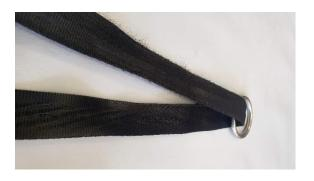
Unacceptable fraying – heavy, causing pulls and deformations in the material.
