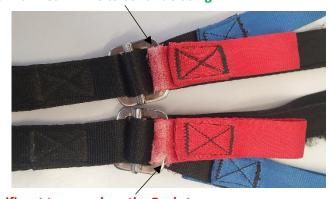
Significant tear -replace the Backstrap
