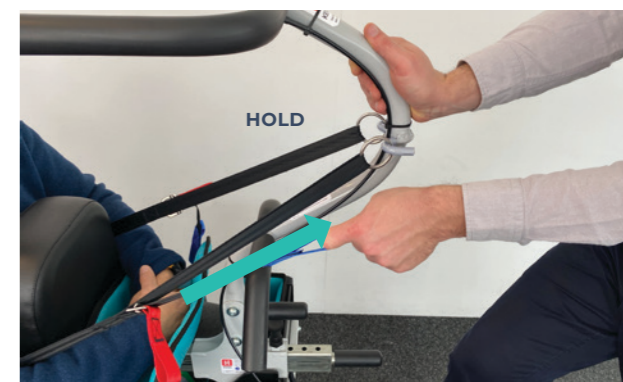
4. One at a time, pull the blue tabs using the technique shown in the photo to ensure suitable tightness (see the next section for tightening tips)
