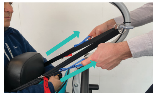
3. Pull both blue tabs at once to evenly tighten the straps
